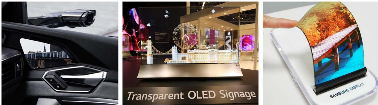
**Figure 2.** OLED applications: replacement of the side-view mirror by an OLED display (left, copyright: Audi AG),<sup>[19]</sup> transparent display (center, copyright: LG Display),<sup>[15]</sup> flexible display (right, copyright: Samsung).<sup>[16]</sup>
