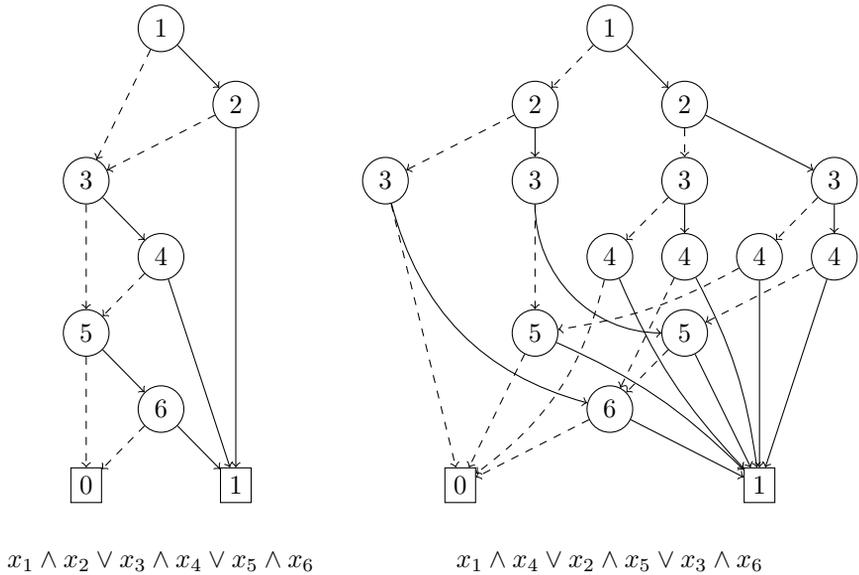
Figure 2.11: Binary Decision Diagrams of two equivalent Boolean functions with different argument ordering
