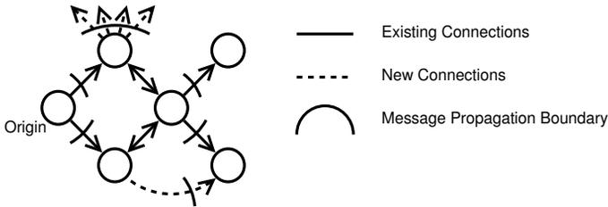
Figure 6.4: Sample network with message propagation boundaries
