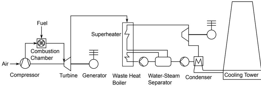
Figure 2.4: Schematic view of a combined gas and steam power plant
