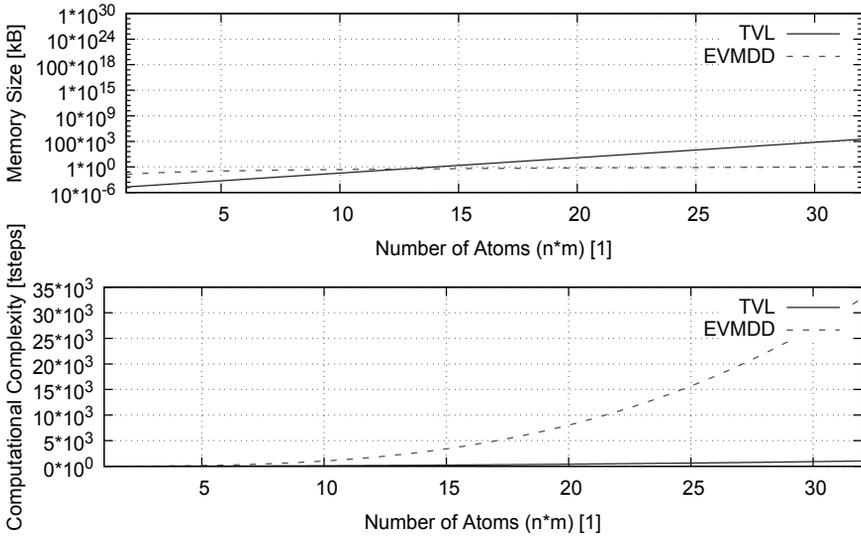
Figure 7.4: Memory size and computational complexity of XBOOLE-based and Edge-Valued Multi-valued Decision Diagram-based demand-supply solvers
