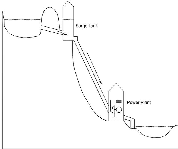
Figure 2.2: Schema of a storage power station
