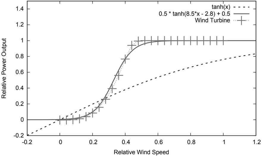
Figure 5.8: The Artificial Neural Network’s activation function and the power curve of a wind turbine
