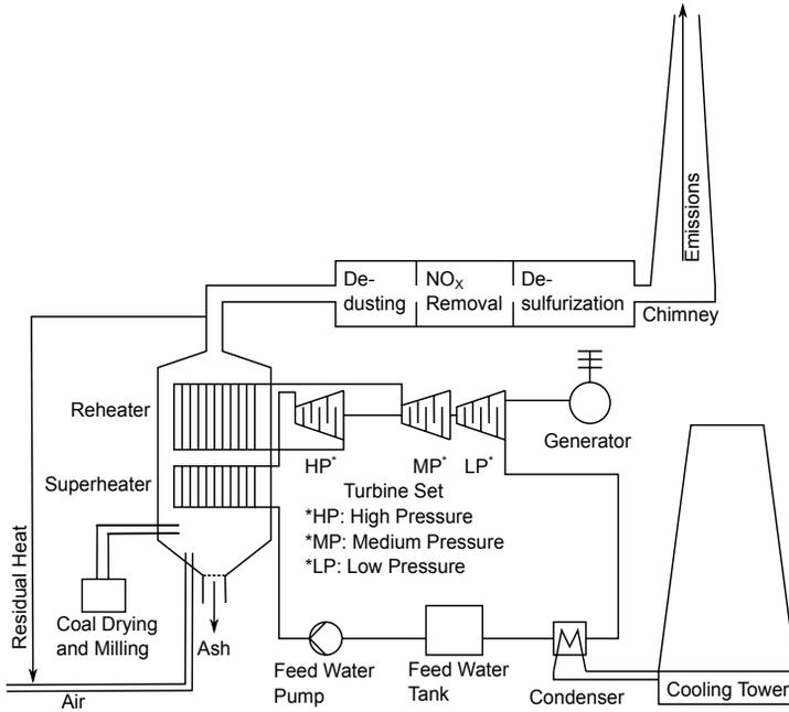
Figure 2.3: Schematic view of a coal power plant
